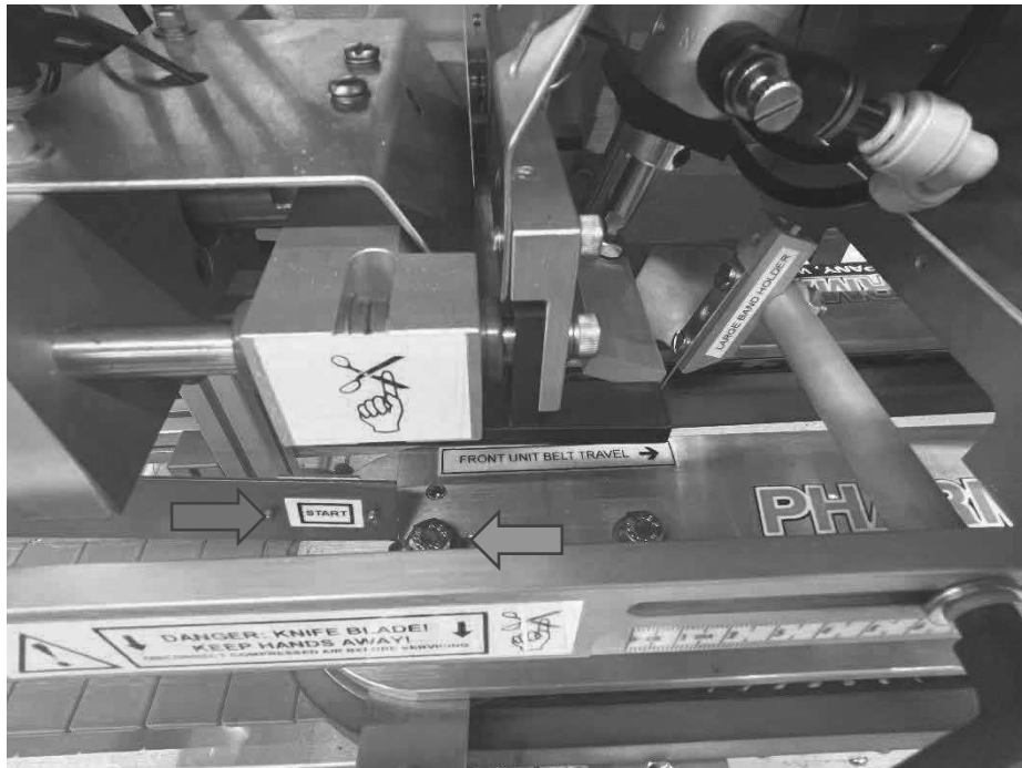
Fig.2: Typical placement of NB1 Start Sensor (blue) at BCV2 Front Belt Tension Screw (green).
