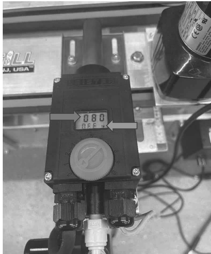
Fig.7: Top number is the actual temperature (red). Bottom number is the called temperature (green).
